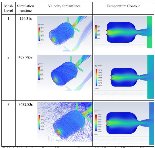
**Table 2**: Velocity Streamlines and Temperature Contours of fuel line and oxidiser line of Vapor Cooled Engine, separated by different mesh size levels
